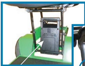
Spare battery under seat
