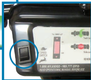
Speed range switch: High speed range 0-4 mph (0-6.4 kph) Low speed range 0-3 mph (0-4.8 kph)
